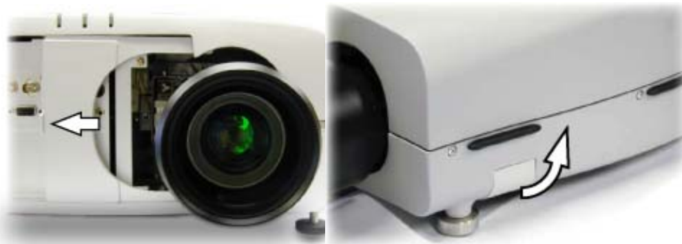
Image 1-2 Release the lens by pulling the unlock handle
