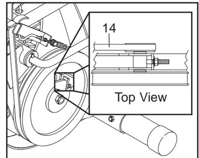
Press down on the center of the Drive Belt (14) between the front and rear pulleys. **There should be from 1/4" to 1/2" of movement in the center of the Belt.** If the Drive Belt (14) is properly adjusted, reattach the side shields and pedals.
