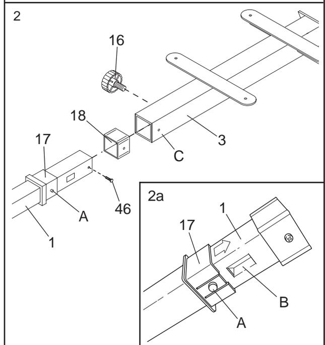
Finally, tighten the Adjustment Knob (16) into the Seat Frame (3).
