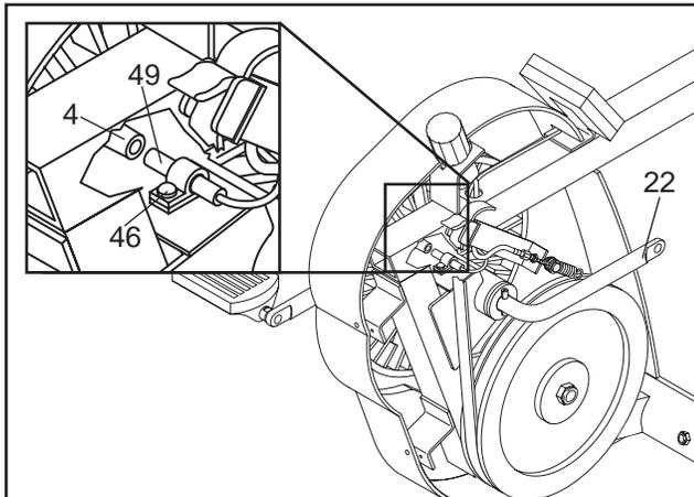
Next, locate the Reed Switch (49). Turn the Crank (22) until the Magnet (4) is aligned with the Reed Switch. Loosen but do not remove the M4 x 16mm Screw (46). Slide the Reed Switch slightly closer to or away from the Magnet. Retighten the Screw. Turn the Crank for a moment. Repeat until the console displays correct feedback. When the Reed Switch is correctly adjusted, reattach the left side shield and pedal.
