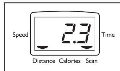
will show that the scan mode is selected, and a flashing mode indicator will show which mode is currently displayed. Note: If a different mode is selected, you can select the scan mode again by repeatedly pressing the mode button.
