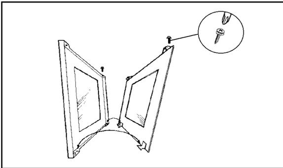
3. Hold the door glass securely in place with one hand before removing the screws completely with the other hand.
