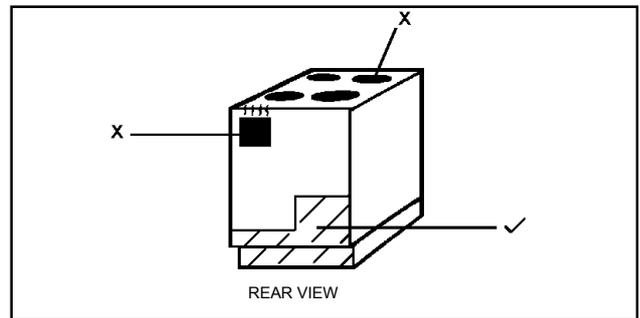
To move the appliance, open the main oven door, and lift the appliance by holding inside the top of the compartment.
