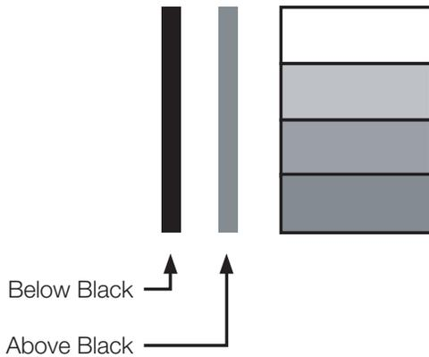
**Figure 4-5. Typical PLUGE Pattern for Adjusting Brightness**
