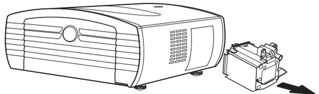
6. Gently slide the new lamp assembly into the lamp cavity. Align the two power connectors at the top of the lamp assembly with the two sockets at the top of the lamp cavity. Press gently on both sides of the lamp assembly to snap it into place. As you do so, the lamp cooling interlock switch returns to the ON position.
