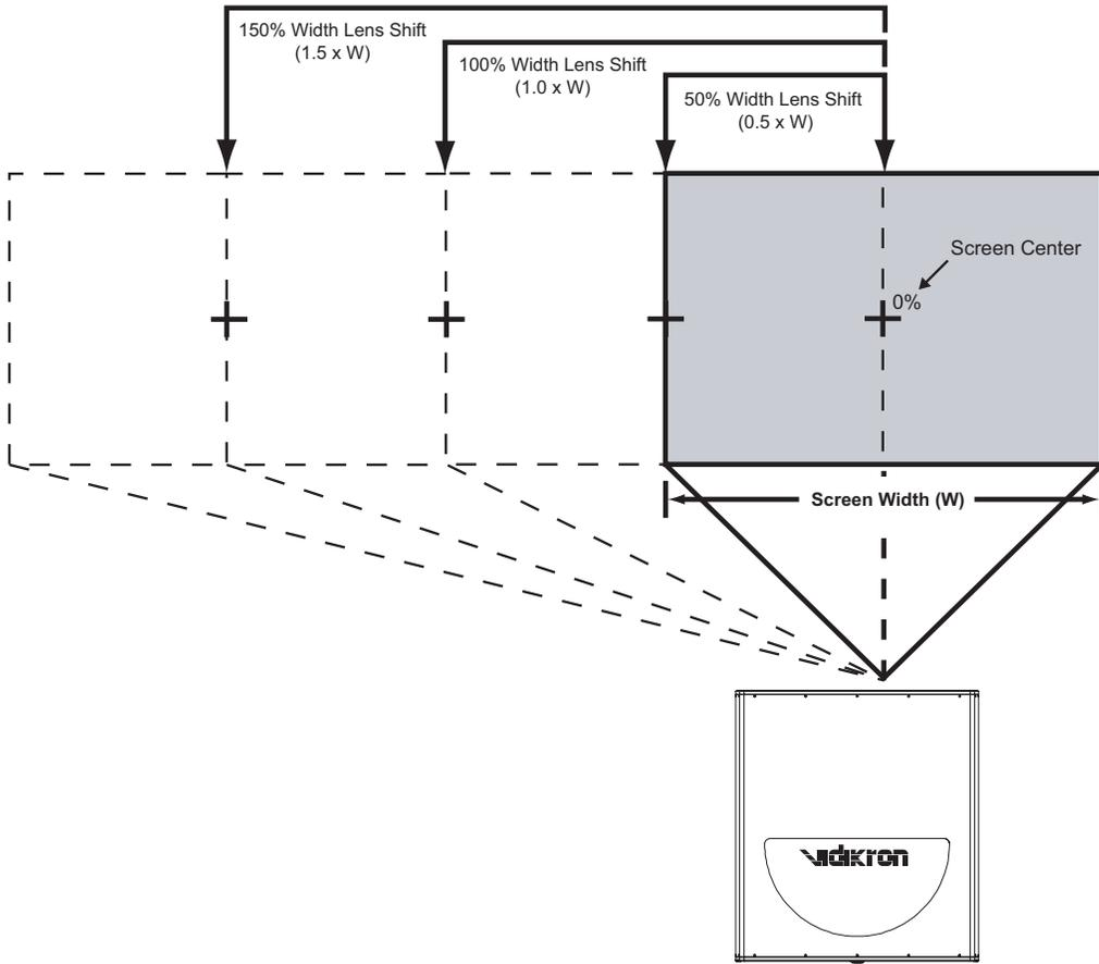
**Note:** This is a general example of lens shift. Lenses vary in their shift capabilities. No particular lens is used in this example.
