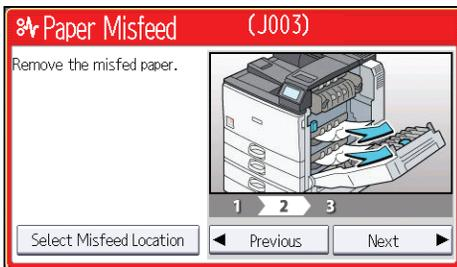
3. When all jammed paper is removed, restore the printer to the original state.
