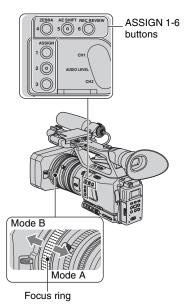
You can adjust the focus manually for different recording conditions.
