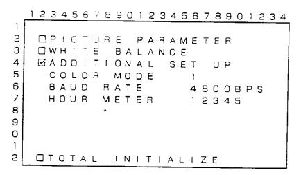
This is common for all input functions. When operating from the remote control unit, select the item to set with the ▲ and ▼ buttons and confirm with the SET button. When operating from the control panel of the Display, select with the + and - buttons and confirm with the SET button.
