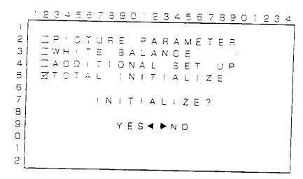
This function resets values adjusted for the Picture Parameters and White Balance back to the factory defaults. Note that this is limited to the data present in the memory area which is currently selected. Select Yes with the doubton on the remote control unit or with the + button on the control panel of the Display to default to the factory set values. Select No with the button on the remote control unit or with the button on the control panel of the Display to reproduce the current state.
