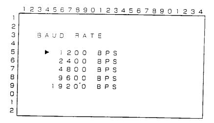
This is common for all input functions. When operating from the remote control unit, select the item to set with the ▲ and ▼ buttons and confirm with the SET button. When operating from the control panel of the Display, select with the + and − buttons and confirm with the SET button. By performing this operation, you can switch the baud rate of the RS232C external control.
