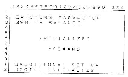
This is the function to reset the adjusted values to the factory defaults. Note that this is limited to the data present in the memory area which is currently selected. Select Yes with the  $\prec$  button on the remote control unit or with the + button on the control panel of the Display to default to the factory set values. Select No with the  $\succ$  button on the remote control unit or with the  $\succ$  button on the control panel of the Display to reproduce the current state.
