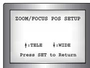
• **ONE PUSH :** Focus is automatically adjusted just once, after zoom position is changed. Select 'ONE PUSH' and press the SET button to confirm. Increase or decrease optical zoom (ZOOM) or digital zoom (D-ZOOM) positions using the directional buttons while verifying the changes on screen. Press the SET button once desired image quality is obtained.
