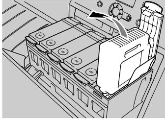
Place the removed ink tank in a vinyl or plastic bag and seal it.
