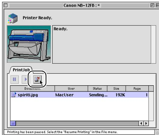
The print queue halts and shifts from the Sending status to the Send status. A red mark is displayed on the right while the print queue is halted.
