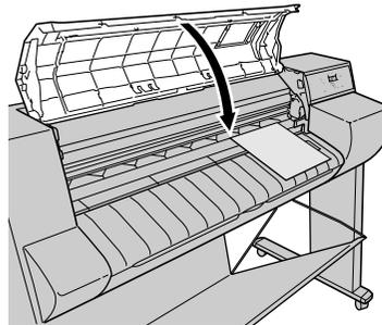
Cut sheet preparation begins. When preparation is finished, the printer is ready to print.
