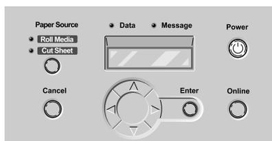
The Online lamp and Message lamp flash for a few seconds while the printer warms up. After the printer has warmed up, if media is loaded in the printer the Online lamp lights and remains on, and “Online” is displayed. The printer is ready to print.
