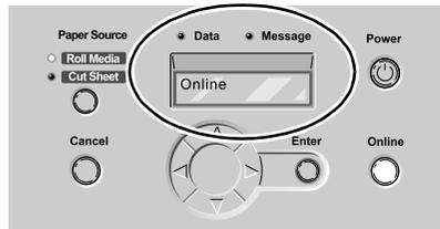
If you see an error message displayed, follow the procedure to correct the problem, and make sure the print job has completed. If a print job is in progress, wait for the print job to complete before switching off the printer.
