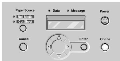
If no print media is loaded in the printer when the printer is switched on, “Offline” is displayed and the printer waits for you to load media in the printer.
