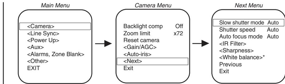
Slow shutter mode slows the frame rate, producing a digital color picture sensitive to low light conditions. The picture may appear rough or smeared, depending on the distance and motion of the viewed image.
