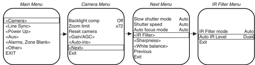
The IR level setting determines when the IR filter will switch IN or OUT. Following are the available settings for the Auto IR Level:
