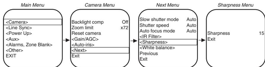
Do the following to manually adjust the sharpness of the picture:
