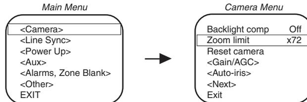
The Spectra II is a 72X zoom camera (18X optical zoom and 4X electronic zoom) can be set for 18X, 36X, 54X, or 72X.
