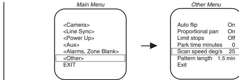
The scan speed is adjustable from 1-40 degrees per second. This occurs in three scan modes: auto, random, and frame scan.
