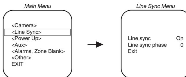
If cameras are out of phase with each other, they may produce what appears to be vertical roll when switching between cameras.
