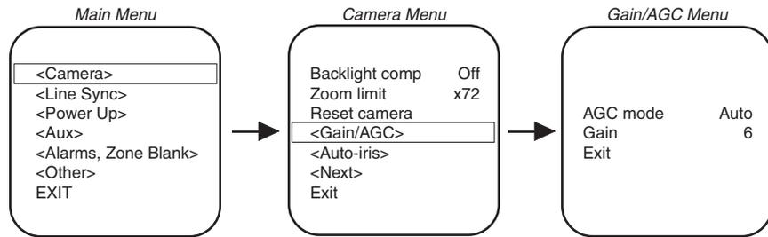
Gain - The amount of amplification the camera places on its video information in order to obtain a full 1-volt peak-to-peak video signal out.
