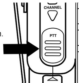
\*\*Note: While the PTT button is depressed, you cannot receive transmissions. The (RX) icon is displayed when the radio is in receive mode.
