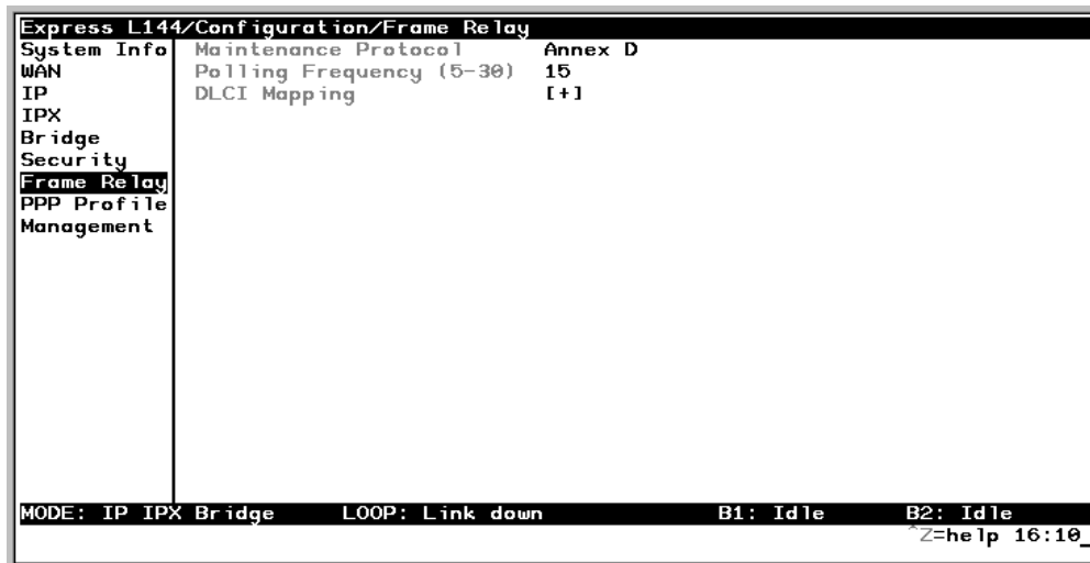
Figure F-01 Configuration/Frame Relay Screen
