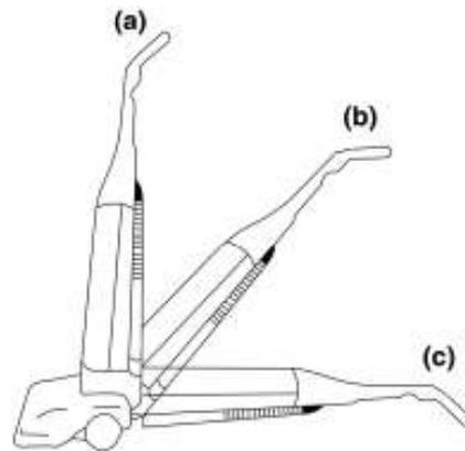
To tilt the vacuum cleaner from the upright position press the handle release pedal with your foot and pull back on the handle.
