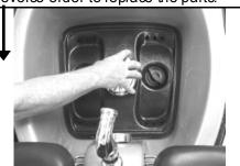
Press firmly down on footplate to help seal while simultaneously tightening tee knobs.
