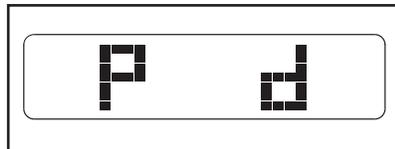
in a store. While the demo mode is turned on, the console will function normally when you plug in the power cord, switch the reset/off circuit breaker to the reset position, and insert the key into the console. However, when you remove the key, the displays will remain lit, although the buttons will not function. If the demo mode is turned on, a "d" will appear in the upper display while the information mode is selected. To turn on or turn off the demo mode, press the Speed decrease button.
