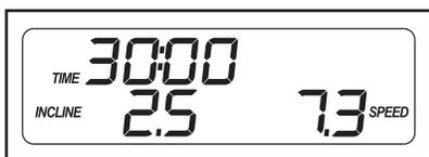
incline setting of the workout will flash in the lower display for a few seconds. In addition, the duration of the workout will appear in the display and a profile of the speed settings of the workout will scroll across the upper display.
