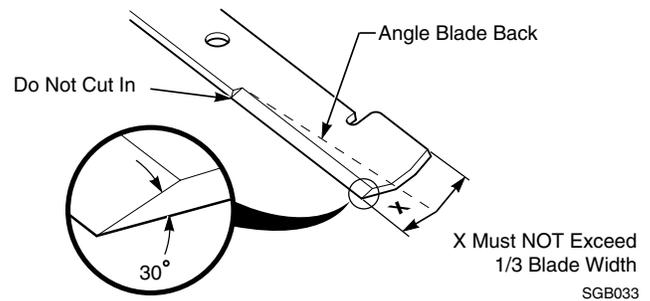
**Figure 7-6. Blade Sharpening**
