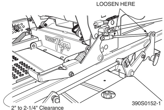
**Figure 6-1. Brake Adjustment**
