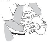
Tightening torque for the bolt holding the blade is: 15-25 Nm (130-215 in.lb).
