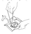
• Undo the screw in the centre of the pulley and remove the pulley. Insert and fasten a new starter cord to the pulley. Wind approx. 3 turns of the starter cord onto the pulley. Connect the pulley to the recoil spring so that the end of the spring engages in the pulley. Fit the screw in the center of the pulley. Insert the starter cord through the hole in the starter housing and the starter handle. Make a secure knot in the end of the starter cord.
