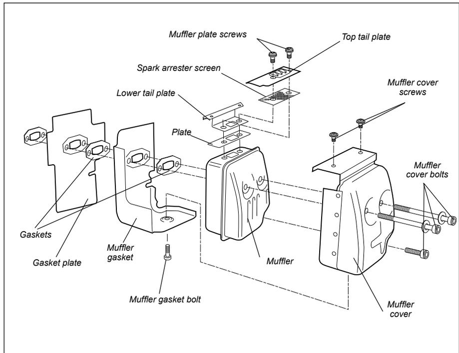
9. Remove the spark arrester screen and clean with a stiff bristle brush.
