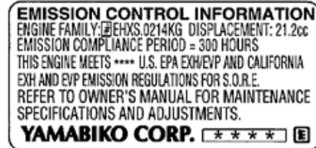
**An Emission Control Label** is located on the unit. (This is an EXAMPLE ONLY; information on label varies by engine FAMILY).
