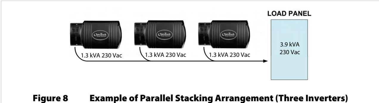
**Figure 8 Example of Parallel Stacking Arrangement (Three Inverters)**
