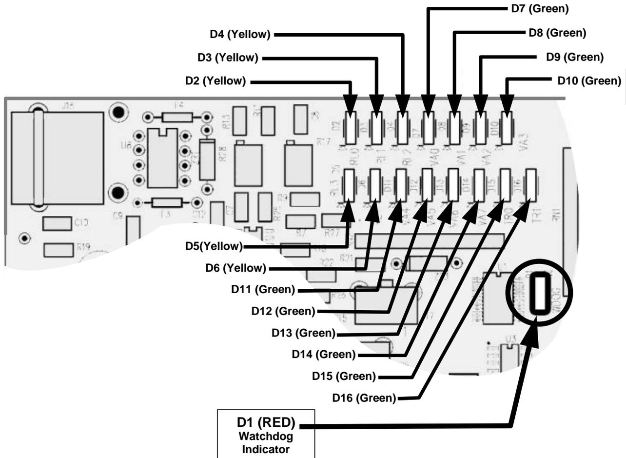
Figure 2-6: Status LED Locations – Relay PCA 04523
