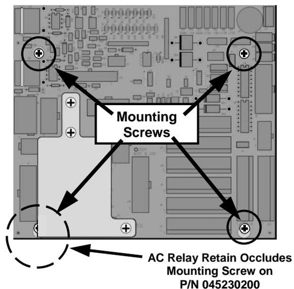
Figure 3-1: Relay PCA 04523 Mounting Screw Locations
