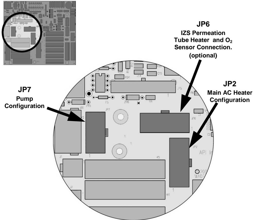
**Figure 2-2: Location of AC power Configuration Jumpers**
