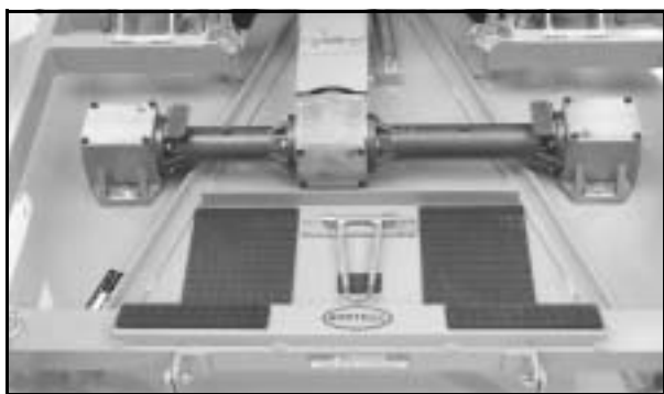
Mower Deck Gearboxes (Shown with Gearbox Cover Removed for Clarity)
