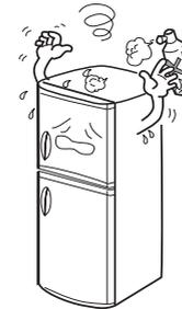
Don't place electrical plugs, regulators or microwaves on top of the refrigerator. Don't use electric appliances (except those allowed by manufacturer) inside the refrigerator.
