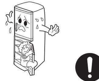
Don't place heavy or unstable articles or water containers on top of the refrigerator.
