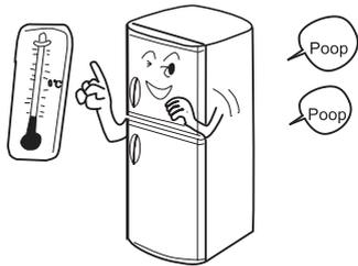
The thermostat, starting capacitor and heat protector may produce a slight sound when the refrigerator is started or closed.
