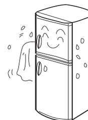
The two sides of the external surface and the middle connection of the refrigerator will be warm due to heat radiation of the appliance.
