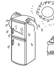
Refrigerator is in direct sunlight, or close to a heat source.
