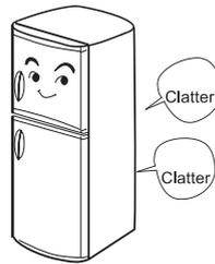
A slight sound may be produced by defrosting water flowing into the evaporating dish and the compressor at the moment of operation commencement or vacation.
