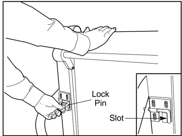
2. Hold the treadmill firmly with both hands, and lower the treadmill to the floor. **To decrease the possibility of injury, bend your legs and keep your back straight.**
