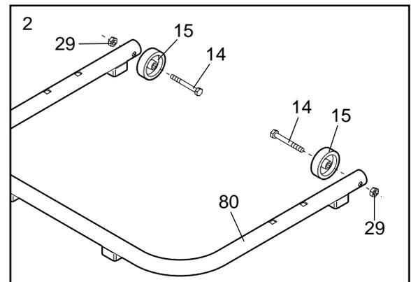
3. With the help of a second person, carefully tip the treadmill onto its left side. Hold the Base (80) against the Right Handrail (6) and the Left Handrail (not shown). **Make sure the Wheels (15) are toward the front of the treadmill as shown.**
