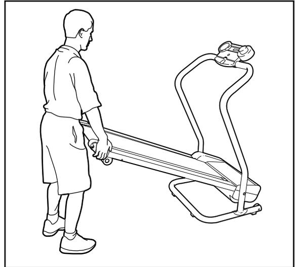
2. Move your right hand to the position shown and hold the treadmill firmly. Raise the treadmill until the latch pin is aligned with the hole in the left handrail. Slide the latch pin into the hole. **Make sure that the latch pin is inserted as far as possible into the hole.** Lock the pin by pressing the end of the pin into the slot in the storage latch as shown in the inset drawing.
