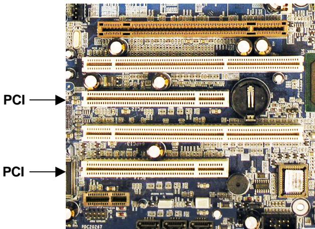
Note: The AD2IDEPRJ Dual Channel IDE JBOD/RAID PCI Controller connects to a PCI Bus slot.
