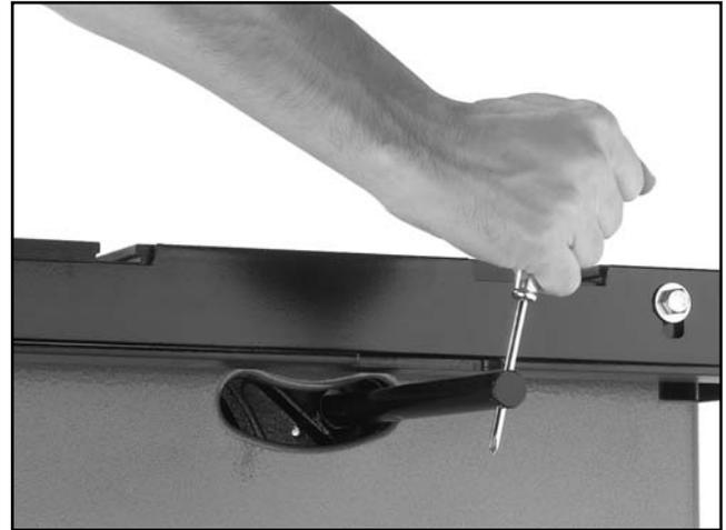
**Figure 12.** Attaching guard support shaft.
