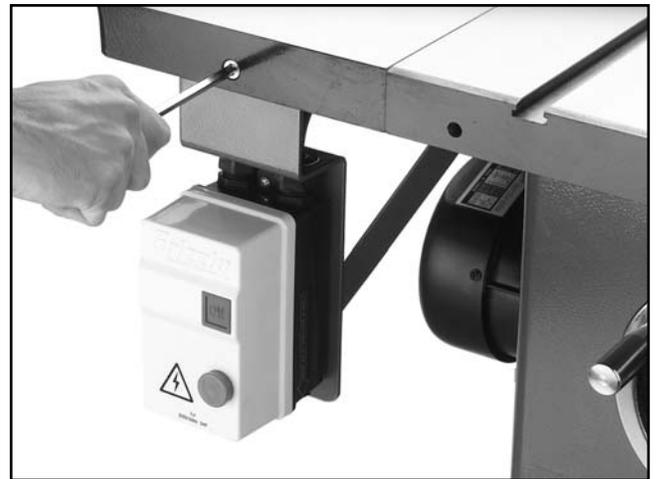
**Figure 10.** Installing switch.
