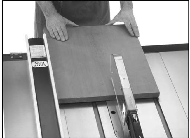
**Figure 37.** Do not stand directly behind wood!
