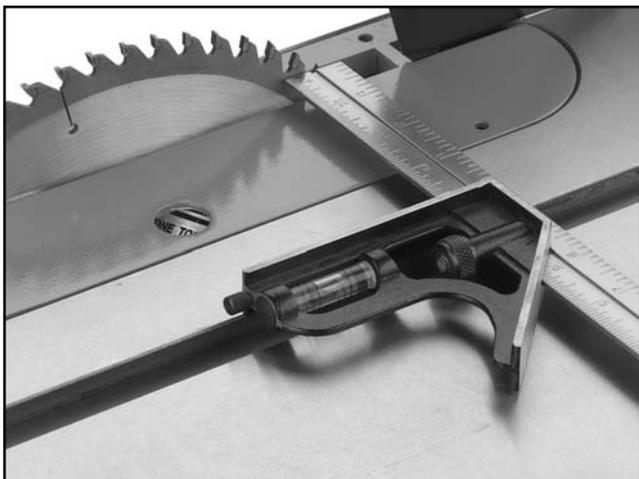
**Figure 24.** Adjusting blade to miter slot.
