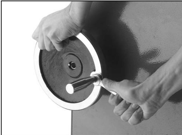
Figure 14. Installing handle on handwheel.
