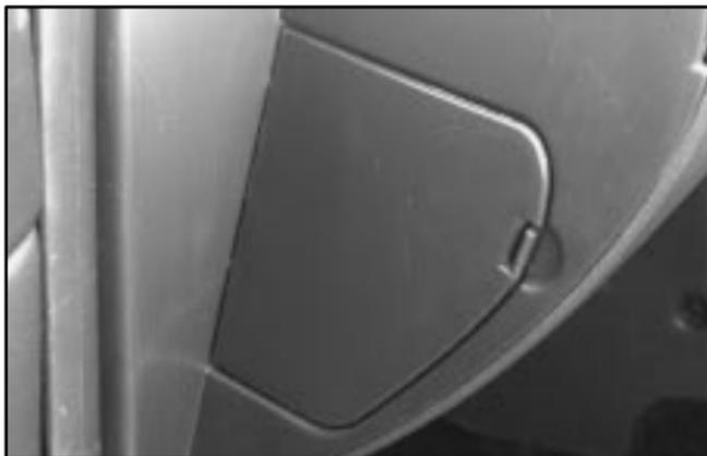
The fuse panel is located at the left end of the instrument panel. To open, push the tab on the access door to the left and pull the door forward. Make sure to insert the tabs when replacing the cover.
