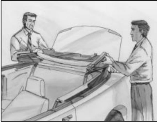
8. Raise the top until it is all the way up. Line up the top so the pins are even with the holes.
