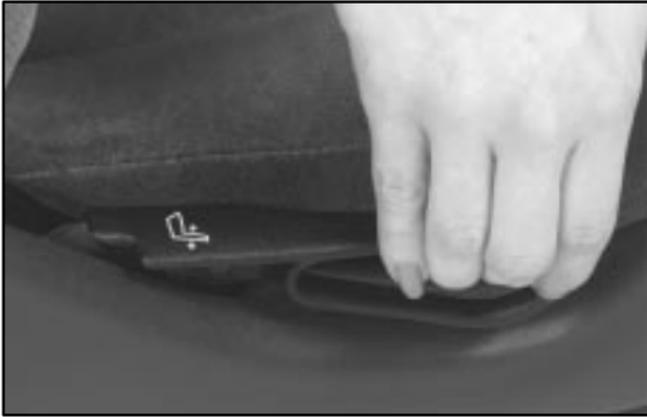
To adjust the seatback, lift the lever on the outer side of the seat and move the seatback to where you want it. Release the lever to lock the seatback. Pull up on the lever and the seat will go to an upright position.
