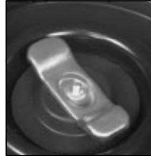
Turn the wing bolt counterclockwise and remove it. Then lift off the adapter and remove the spare tire.
