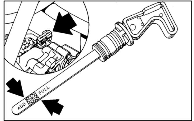
3. Check both sides of the dipstick and read the lower level. The fluid level must be between the ADD and FULL marks. (Note: Fluid may appear at the bottom of the dipstick even when the fluid level is several pints low.)
