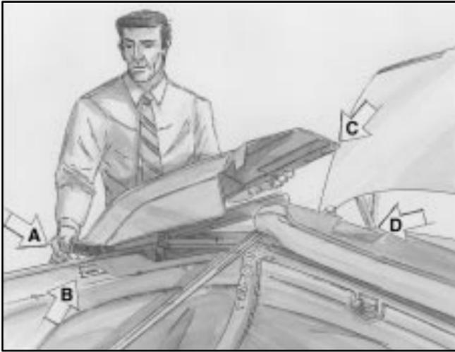
3. Install the boot side cover by inserting the tab (A) on the underside of the cover into the slot (B) at the top of the quarter trim panel. Place the rear flap of the boot side cover in the trunk lid opening, aligning the eyelet (C) over the boot snap ball stud (D).
