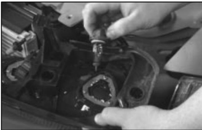
3. Disconnect the bulb base from the socket by lifting the plastic locking tab.
