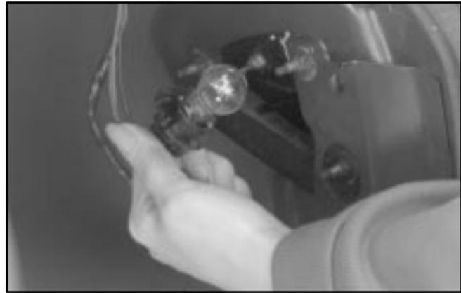
3. To remove the bulb, pull it out.
