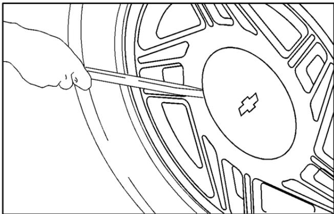
2. On some models, a cover plate must be removed to find the wheel nuts. Carefully use the wedge end of the wheel wrench to pry it off.
