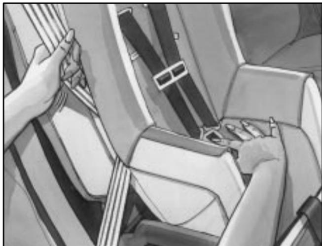
5. To tighten the belt, pull up on the shoulder belt while you push down on the child restraint. If you're using a forward-facing child restraint, you may find it helpful to use your knee to push down on the child restraint as you tighten the belt.
