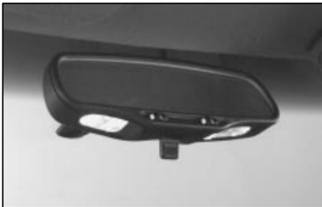
These lamps are located on the rearview mirror. Turn each one on and off by pressing its switch.
