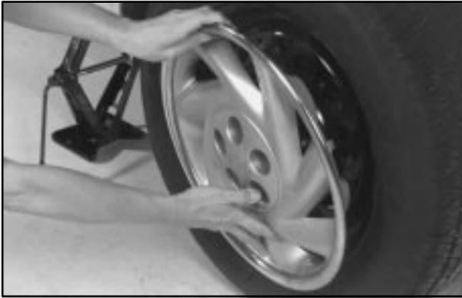
7. If you have a wheel cover, use your fingers to carefully pull the wheel cover from the wheel. Then remove the flat tire.
