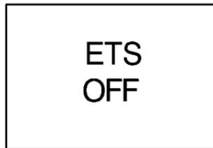
With the Enhanced Traction System (ETS), this warning light should come on briefly as you start the engine.
