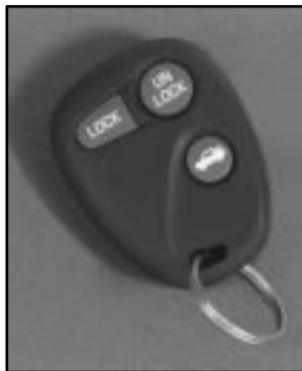
The remote keyless entry system consists of a receiver, which is located in the vehicle, and two hand held transmitters.
