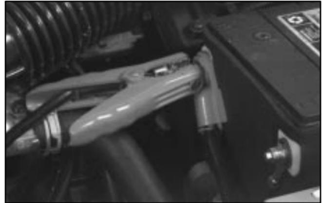
7. Remove the red plastic cap, and connect the red positive (+) cable to the positive (+) terminal of the vehicle with the dead battery. Use a remote positive (+) terminal if the vehicle has one.
