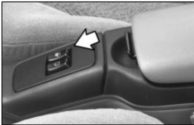
With power windows, switches on the center console control each of the windows when the ignition is on. In addition, on four-door models, each rear passenger door has a control switch for its own window.
