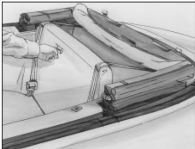
1. From inside the vehicle, pull the tab on the rear seat to fold down the seat. See “Fold-Down Rear Seat” in the Index.
