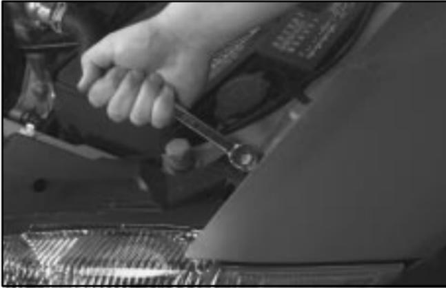
1. Remove the first bolt. Then remove the remaining plastic fasteners holding the shield. Use the end of a flat-head screwdriver to pull up the center of the fastener. Be careful not to break the fasteners that hold the shield in place.
