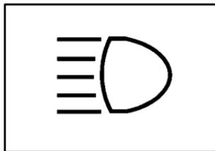
When the high beams are on, this light on the instrument panel will also be on.
