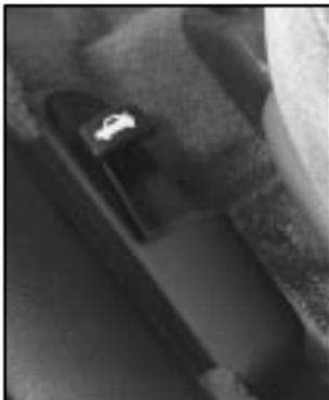
Pull upward on the remote release handle, located on the floor near the left side of the driver's seat, to release the trunk lid.
