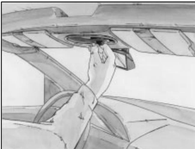
6. Turn the latch handle up to lock the top. Be sure the top is securely latched on both sides.
