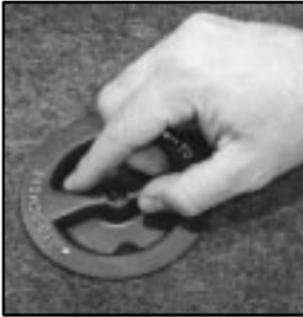
The equipment you'll need is in the trunk. Turn the center retainer nut on the compact spare cover counterclockwise to remove it.
