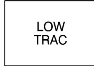
When your Enhanced Traction System is limiting wheel spin, this light will come on.
