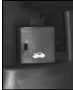
To open the hood, first pull the handle inside the vehicle on the driver's side under the instrument panel.
