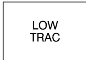
This light will come on when your Enhanced Traction System is limiting wheel spin. See “Enhanced Traction System Active Light” in the Index.
