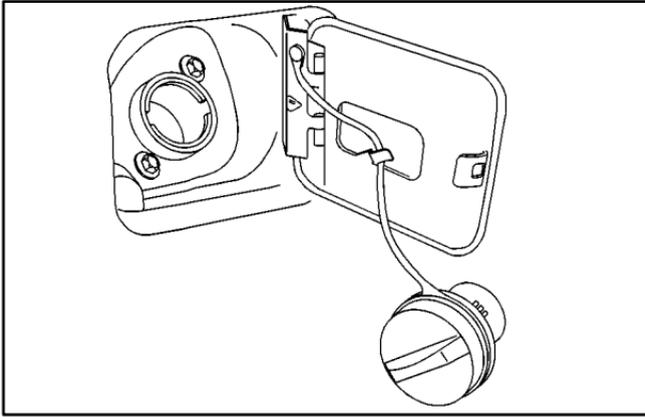
While refueling, hang the tethered cap inside the fuel door by placing the fuel cap strap in the strap hanger.
