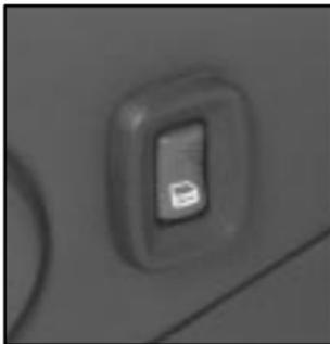
You can lock or unlock all doors of your vehicle from the driver's or front passenger's door lock switch.
