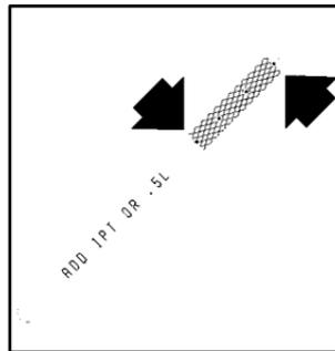
3. Check both sides of the dipstick, and read the lower level. The fluid level must be in the cross-hatched area.
