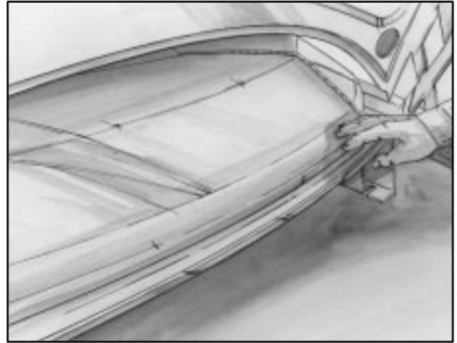
6. Go to the rear of the vehicle. Place the boot center cover along the trunk lid opening. Align one snap on the corner of the boot to the ball stud and push forward. Repeat for other snap.
