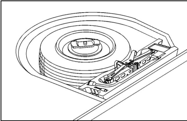
Remove the jack and wheel wrench from the trunk. Your vehicle's jack and wheel wrench are stored in a foam tray. Remove the band around the jack.
