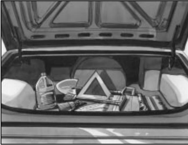
Include an ice scraper, a small brush or broom, a supply of windshield washer fluid, a rag, some winter outer clothing, a small shovel, a flashlight, a red cloth and a couple of reflective warning triangles. And, if you will be driving under severe conditions, include a small bag of sand, a piece of old carpet or a couple of burlap bags to help provide traction. Be sure you properly secure these items in your vehicle.
