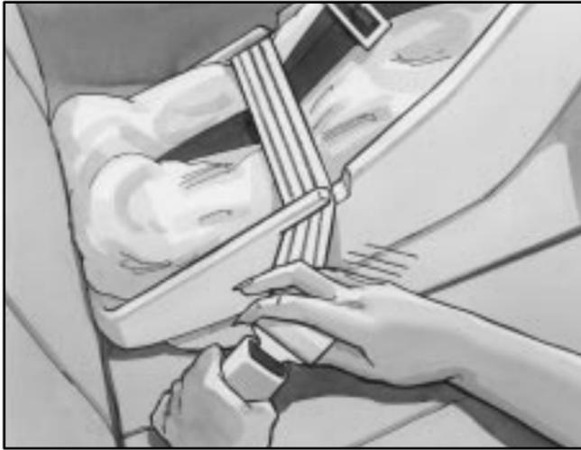
4. Buckle the belt. Make sure the release button is positioned so you would be able to unbuckle the safety belt quickly if you ever had to.
