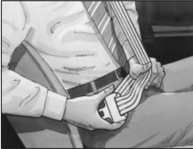
If the belt stops before it reaches the buckle, tilt the latch plate and keep pulling until you can buckle the belt.
