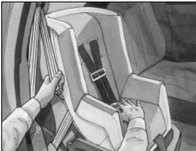
6. To tighten the belt, pull up on the shoulder belt while you push down on the child restraint. You may find it helpful to use your knee to push down on the child restraint as you tighten the belt.
