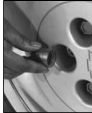
1. Using the wheel wrench, remove the plastic nut caps (if equipped).
