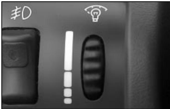
You can brighten or dim the instrument panel lights by turning the dial up or down.
