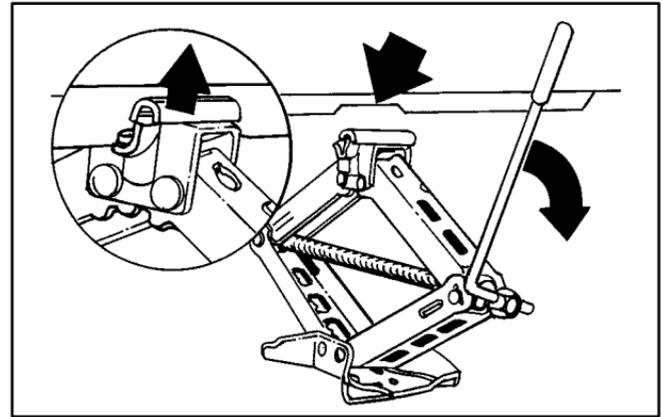
5. Raise the vehicle by turning the jack handle clockwise. Raise the vehicle far enough off the ground so there is enough room for the spare tire to fit.
