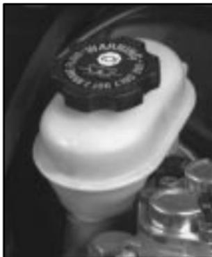
Your brake master cylinder reservoir is on the driver's side of the engine compartment. It is filled with DOT-3 brake fluid.
