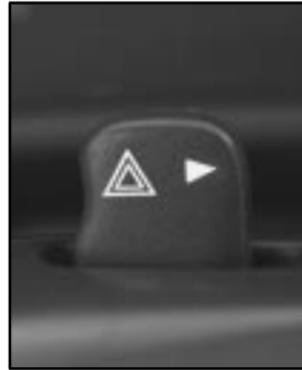
Move the switch to the right to make your front and rear turn signal lamps flash on and off.
