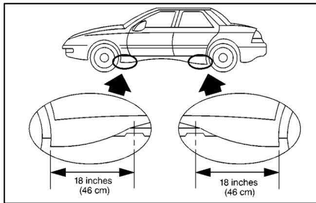
4. Near each wheel well is a notch in the frame which the jack head fits in. The front notch is 9 inches (23 cm) back from the front wheel well. The rear notch is 8 inches (20 cm) forward from the rear wheel well. As is shown in the diagram above, if your vehicle has flared side moldings, both front and rear notches are 18 inches (46 cm) from the wheel wells.
