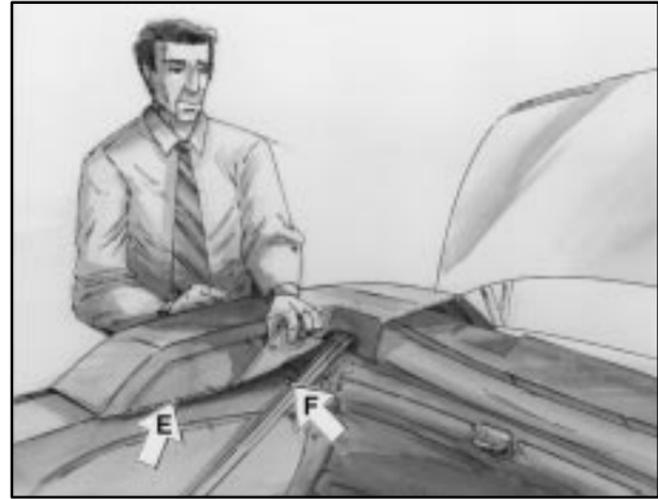
4. Attach the two snaps on the inside flap of the side cover to the top of the quarter trim panel. Attach the front snap (E) first and then the rear snap (F). The rear snap is adjustable for ease of installation.
