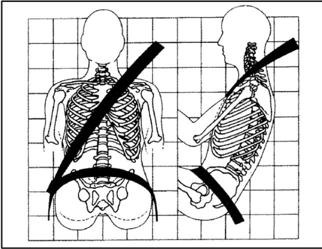
The lap part of the belt should be worn low and snug on the hips, just touching the thighs. In a crash, this applies force to the strong pelvic bones. And you'd be less likely to slide under the lap belt. If you slid under it, the belt would apply force to your abdomen. This could cause serious or even fatal injuries. The shoulder belt should go over the shoulder and across the chest. These parts of the body are best able to take belt restraining forces.
