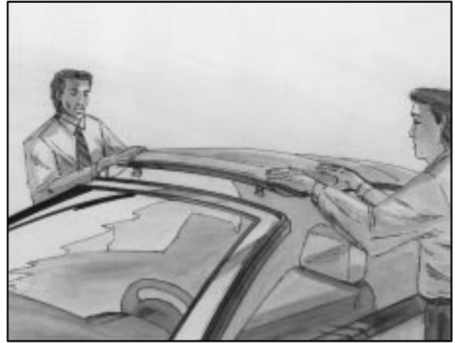
9. Pull down on the top and rotate the latch handle up to lock the convertible top. Be sure the top is latched securely on both sides.
