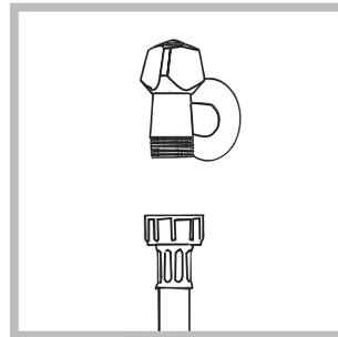
1. Connect the supply pipe by screwing it to a cold water tap using a 3/4 gas threaded connection (see figure). Before performing the connection, allow the water to run freely until it is perfectly clear.
