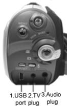
**3. Audio plug** – The audio plug connects the headphone. Listen to music on the digital video camera. At the same time, this can function as audio input/output plug. Note: if using the radio function, the headphones have to be plugged in to function as antenna to receive radio channels.
