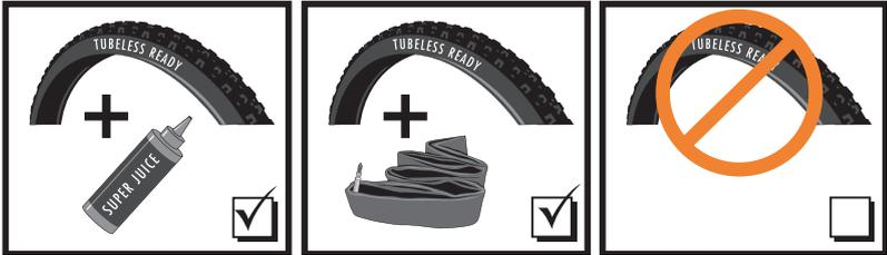
Tubeless Ready tires do not hold air without either an inner tube or liquid sealant inside the tire. To use a Tubeless Ready tire in tubeless mode, follow these instructions to install Bontrager Super Juice sealant. Super Juice is a long-lasting, quick-acting, glycol-based sealant developed for this purpose.
