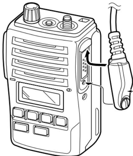
**CAUTION:** Attach the speaker-microphone's connector securely to prevent accidental dropping, or water intrusion in the connector.
