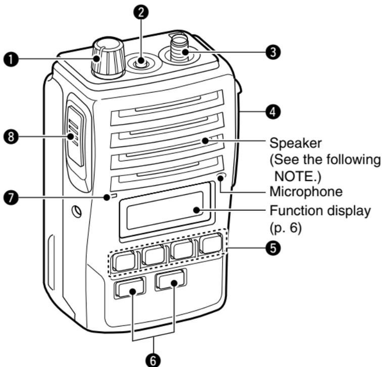
**NOTE:** If the speaker netting (for dust proofing) becomes wet, dry it with a hair drier (cool mode) etc. before operating the transceiver. Otherwise the audio may be difficult to hear for loss of the sound pressure.
