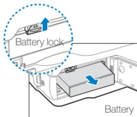
Push the lock up to release the battery.
