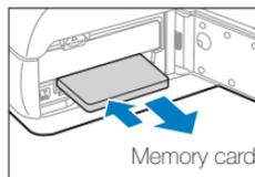
Push gently until the card disengages from the camera and then pull it out of the slot.
