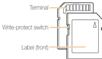
You can prevent files from being deleted by using a write-protect switch on the SD or SDHC card. Slide the switch down to lock or slide it up to unlock. Unlock the card when shooting.
