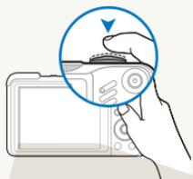
Half-press **[Shutter]** and adjust the focus. Focus and exposure will be adjusted automatically.
