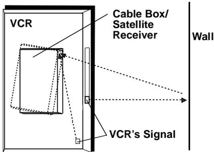
To help the VCR's signal reach your cable box or direct-to-home satellite receiver, place the VCR and your equipment near each other. You might also have to adjust the position of your cable box or direct-to-home satellite receiver as shown above.
