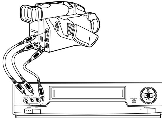
1. Insert the plugs at one end of the cable into the **AV 2 L-AUDIO IN-R** and **AV VIDEO IN** jacks on the front panel. If the camcorder's audio is monaural, connect the audio cable to the **L-AUDIO IN** jack only.
