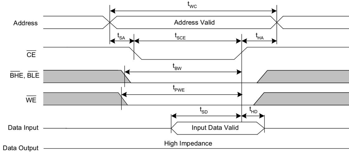
**Figure 11. SRAM Write Cycle 3:  $\overline{\text{BHE}}$  and  $\overline{\text{BLE}}$  Controlled**<sup>[5, 18, 19, 20, 21]</sup>
