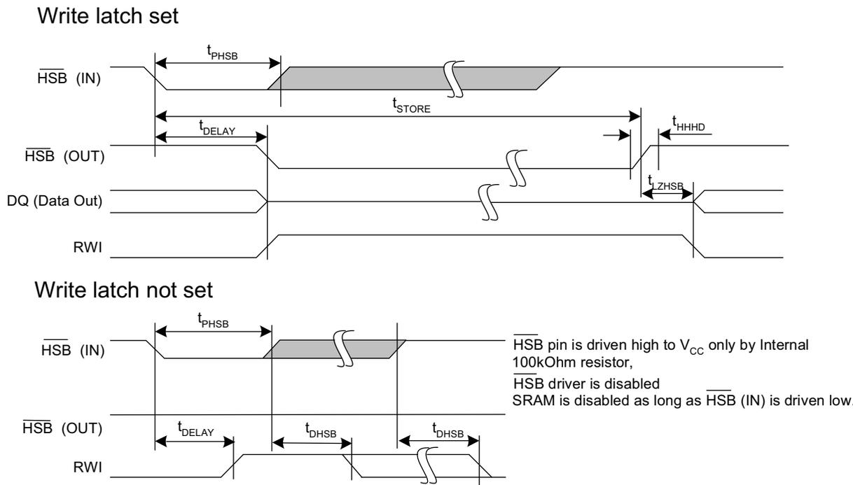
**Figure 16. Soft Sequence Processing<sup>[31, 32]</sup>**
