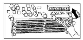
4. Connect the 8-pin or 4+4-pin connector for the CPU. If your motherboard has an 8-pin socket with a cover on some of the openings, we recommend that you remove the cover and use the 8-pin connector.
