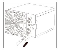
6. Connect the AC power cord to the power supply AC inlet. Be sure to use the heavy-duty cord supplied with your CP-1000.
