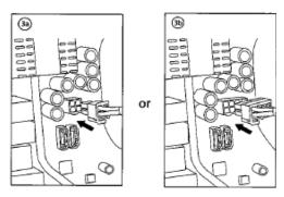
5. Connect extra cables from the cable pack to the sockets on the power supply only if needed. If you are going to plug the PCI-E cables into the PSU, they should go into the red sockets. If the red sockets are not being used for PCI-E, then they can be used for any other type of cable supplied in the pack that accompanies the PSU.
