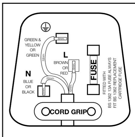
With alternative plugs a 13 A fuse must be fitted either in the plug or adaptor or in the main fuse box. If in doubt contact a qualified electrician.
