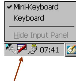
A range of different software keyboards are provided for entering characters on the device. The «**Input Panel active**» setting can be used to activate or deactivate the software keyboard. The option is deactivated by default. A change of this setting requires the system to be restarted.
