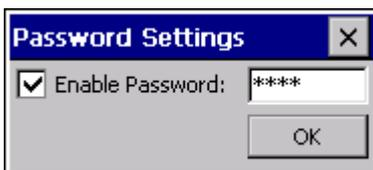
The password settings are stored in the file «CERemoteSvr.ini» in the directory «\Bootdevice\os\». The data stored is naturally encrypted. The file is stored on the Flash card, which means that the password settings are also retained after a restart.
