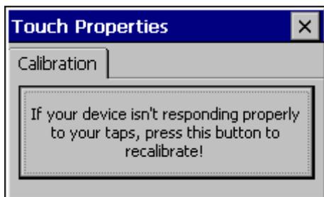
This program is used for the [Touch calibration](#) and for the [Touch Enable/Disable](#). If the program is started without command line parameters, the following dialog appears:
