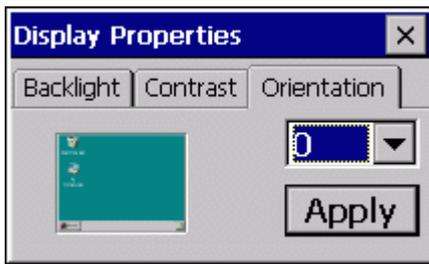
Display orientation can be set with the «0» (default setting) or «90» settings. The display is rotated in a clockwise direction. The «90» setting should be selected for vertical mounting. The picture on the left of the dialog shows the orientation set. The setting is not transferred until after a restart.
