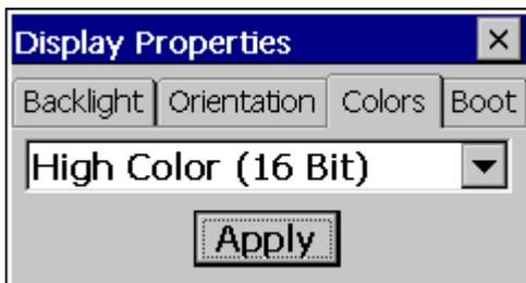
This setting enables the number of screen colors to be selected. Different color depths can be selected. The setting is not transferred until after a restart.
