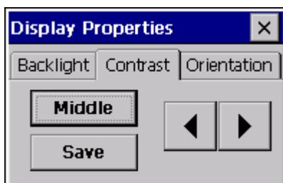
This program is used for setting the screen contrast. The «Middle» setting is the factory setting. Touch «Save» to save the selected setting as persistent data, i.e. the value is retained even after a restart.
