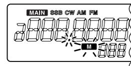
**NOTE:** When SSB, CW, AM, FM, WFM or Digital mode frequencies are programmed into memory channels randomly, memory scan is slow because changing modes takes time. In this case, assign the SSB, CW, AM, FM, WFM or Digital mode frequencies into separate banks where bank scan can be used. And using the bank scan is helpful.
