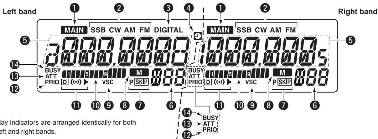
\*Display indicators are arranged identically for both the left and right bands.
