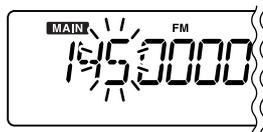
While 1 MHz tuning step is selected, the 1 MHz digit blinks.
