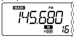
The display shows that memory channel 16 is set as a skip channel.
