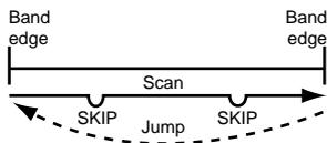
Skips unwanted frequencies or channels that inconveniently stop scanning. This function can be turned ON and OFF by pushing and holding **[SET•SKIP]** in *memory mode*.
