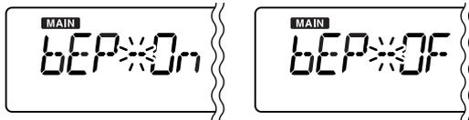
Even when this item is set to OFF, the power-on beep and pocket beep function still sound. The power-on beep can not be set to OFF.
