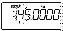
While 10 MHz tuning step is selected, the 10 MHz digit blinks.
