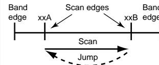
Repeatedly scans between two user-programmed frequencies. Used for checking for frequencies within a specified range such as repeater output frequencies, etc.
