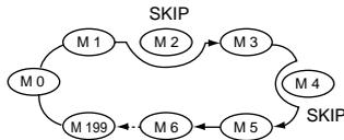
Repeatedly scans memory channels except those set as skip channel. Skip channels can be turned ON and OFF by pushing and holding **[SET•SKIP]** in *memory mode*.
