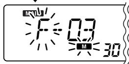
④ Rotate the same band's **[DIAL]** to select the desired bank indicator to transfer or erase.
