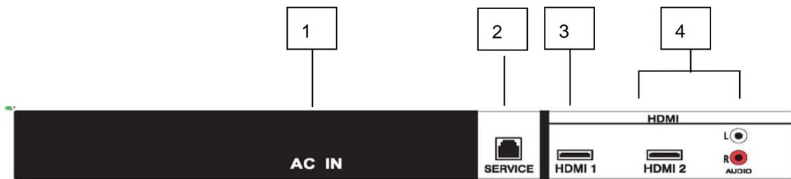
1. **AC IN** – Plug-in the supplied AC Power Cord here.
