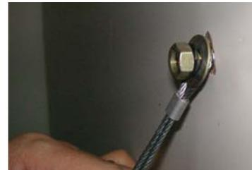
2. Fix the other end of the Safety Strap to one of the upper wall mounting holes on the back of the HDTV, using a washer under the screw head.
