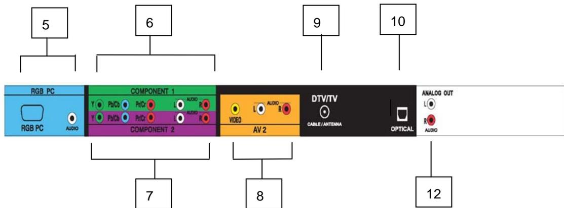
5. **RGB PC** – Connect the video and audio from a computer here. The blue color band on the rear of the TV indicates this connection.
