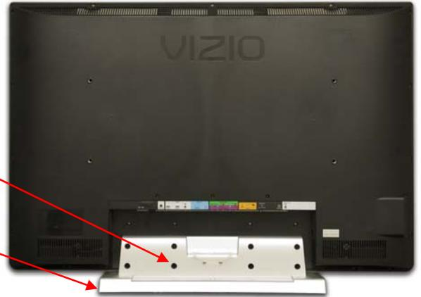
5. Now, the VU42L FHDTV10A can fit securely to a mount (sold separately) by utilizing the mounting holes in the center of the back panel of the TV. Please make sure to read the instructions of your specific mount to properly hang the VU42L FHDTV10A.
