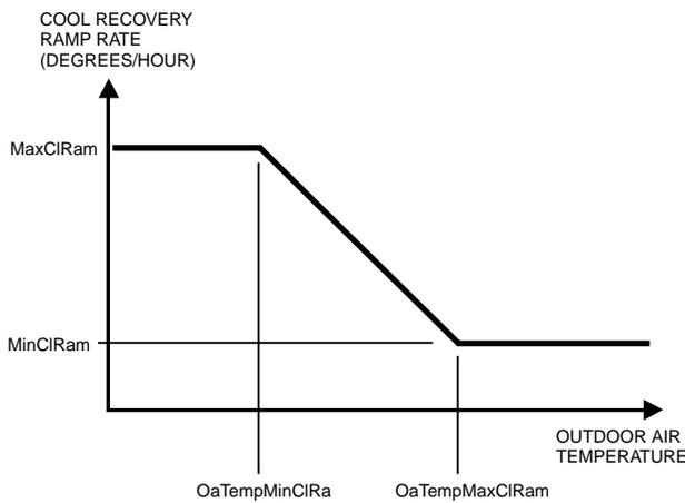
**Fig. 48. Setpoint ramping parameters with ramp rate calculation.** M10111
