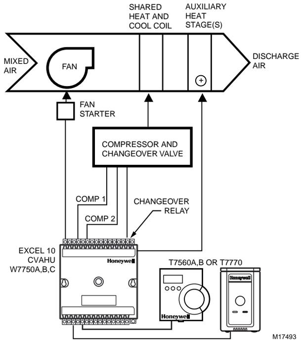
Fig. 15. Heat pump with two compressors and auxiliary heat stage(s).
