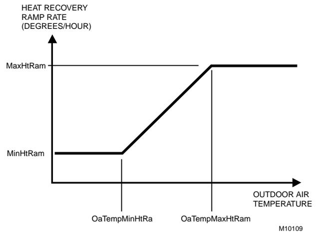
**Fig. 46. Setpoint ramping parameters with ramp rate calculation.**
