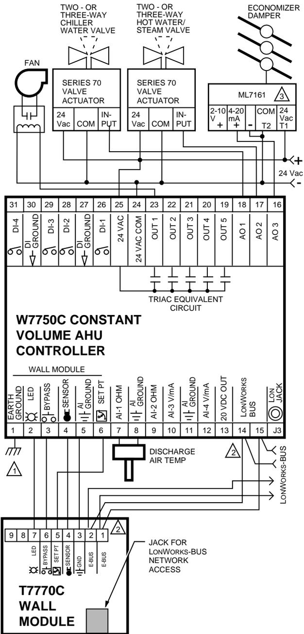
Fig. 35. W7750C Controller with 4-to-20 mA heating, cooling and economizer wiring diagram. AOs must use terminals 16, 17 or 18. The AOs can be set to be reverse acting. (For more information on note 2, refer to Fig. 25.)
