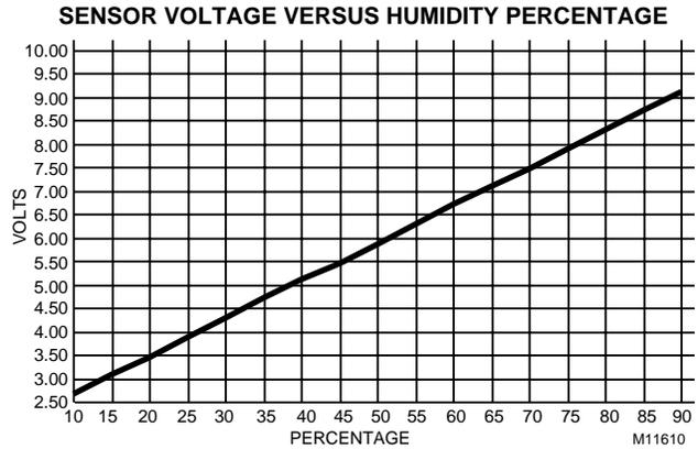
Fig. 57. Graph of Sensor Voltage versus Humidity.
