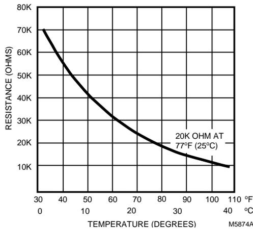
**Fig. 54. Graph of Sensor Resistance versus Temperature.**
