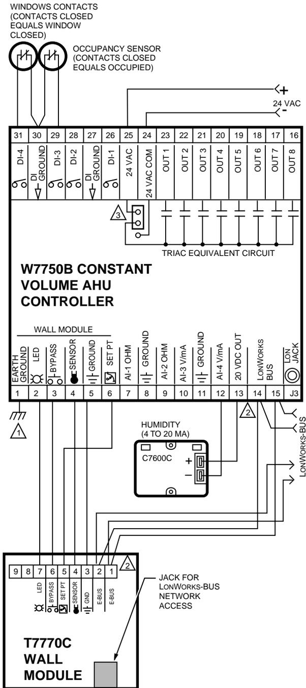
Fig. 34. W7750B,C wiring diagram with C7600C 4 to 20 mA solid state humidity sensor. (For more information on note 2, refer to Fig. 25.)
