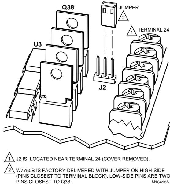
**Fig. 26. W7750B High-Side/Low-Side selectable switching and jumper location.**
