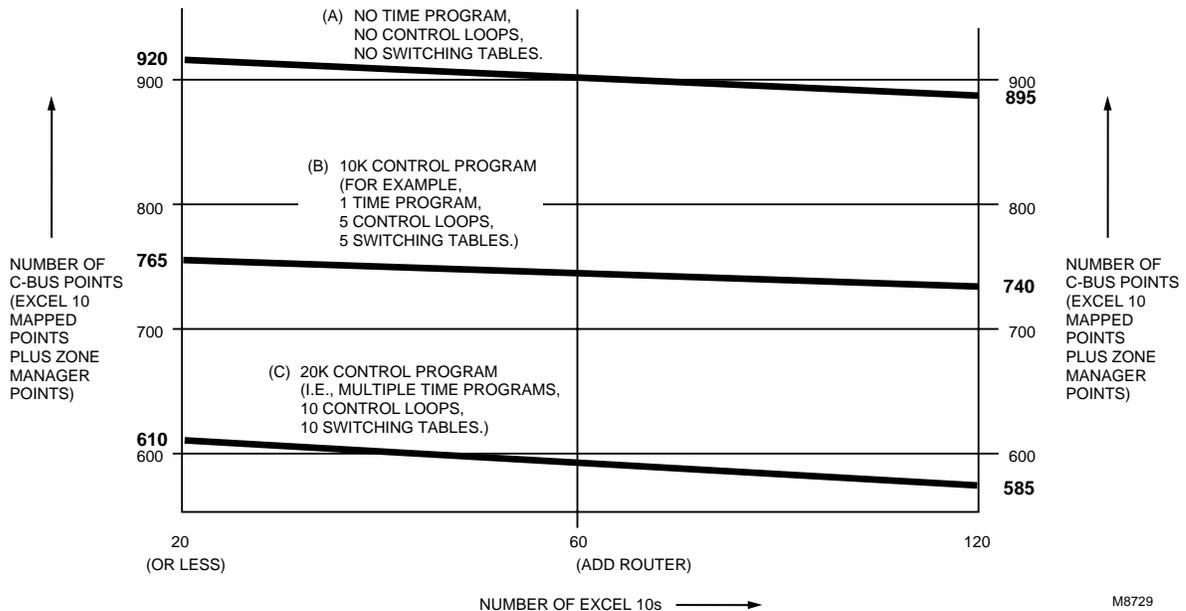
Fig. 51. Point capacity estimate for Zone Manager.
