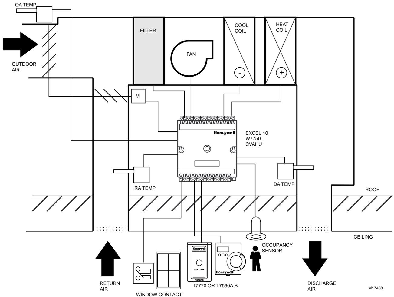
**Fig. 49. Schematic diagram for a typical W7750B Unit.**
