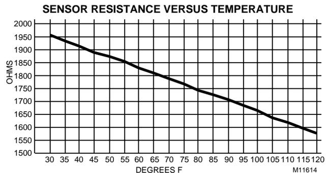
**Fig. 53. Graph of Sensor Resistance versus Temperature.**
