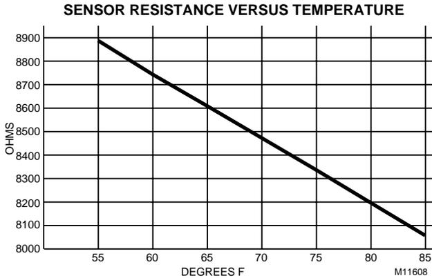
Fig. 56. Graph of Sensor Resistance versus Temperature.
