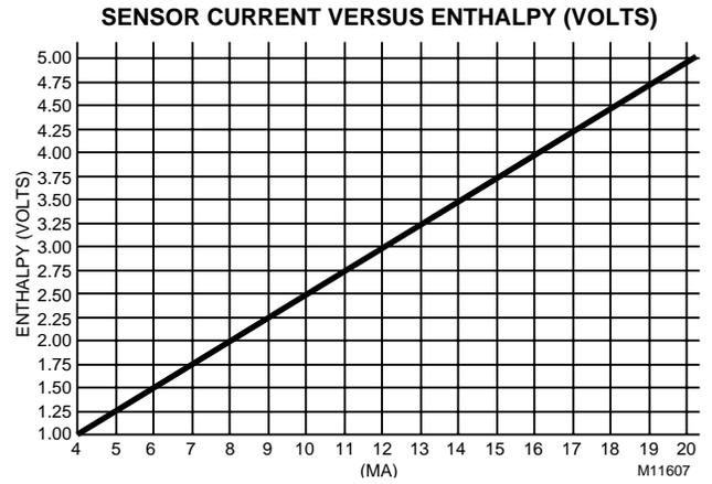
**Fig. 59. Graph of Sensor Current versus Enthalpy (volts).**
