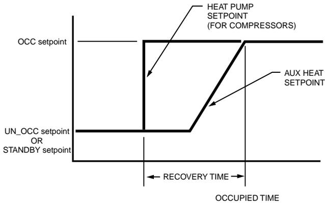
**Fig. 47. Setpoint ramping parameters with setpoint calculation.** M10110
