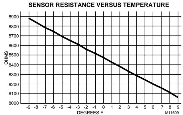
**Fig. 55. Graph of Sensor Resistance versus Temperature.**
