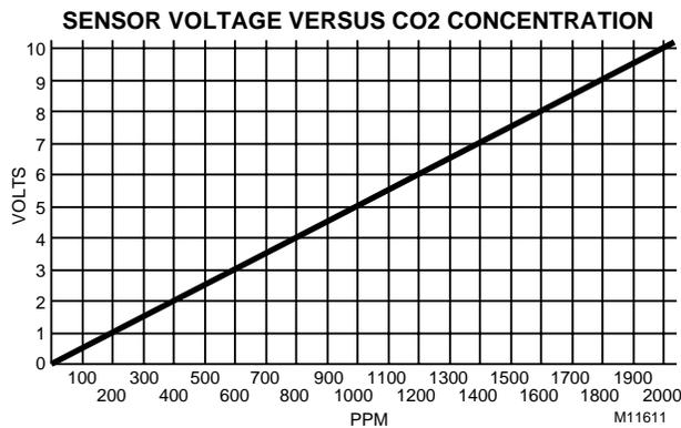
**Fig. 62. Graph of Sensor Voltage versus CO<sub>2</sub> concentration.**
