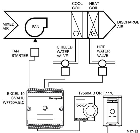
**Fig. 14. Fan, modulating heating and modulating cooling.**
