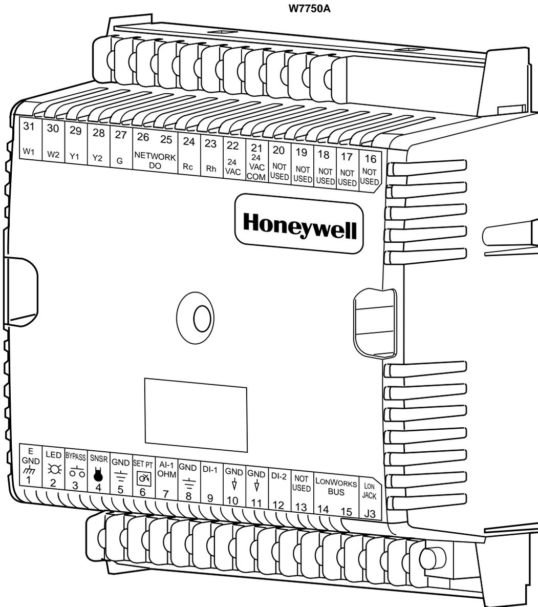
**Fig. 3. Excel 10 W7750A Constant Volume AHU Controller.**
