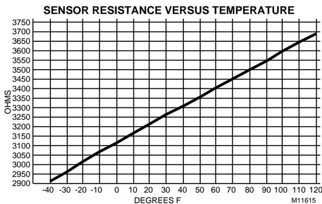
**Fig. 52. Graph of Sensor Resistance versus Temperature.**
