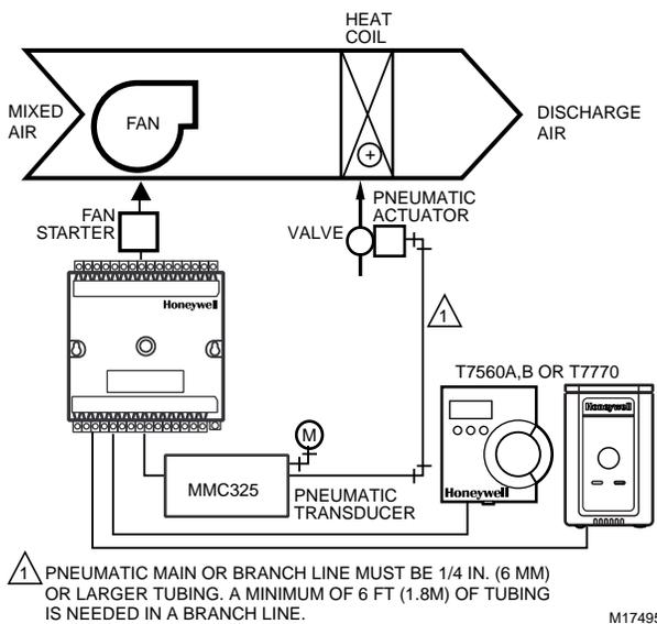
**Fig. 17. Modulating heat with pneumatic valve actuator.**
