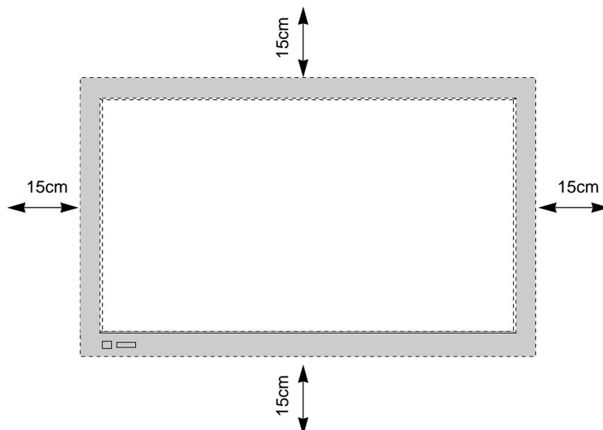
**If proper spacing is not allowed, it may cause the plasma display to overheat, which can cause fire or damage to the unit**
