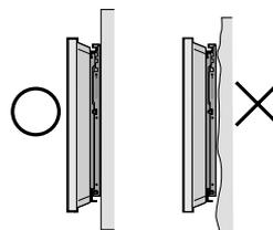
(If attached on an unstable wall, the unit can fall and break)
