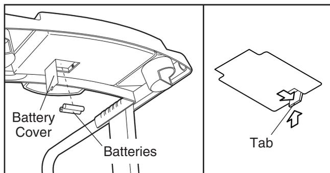
Close the battery cover, push up on the battery cover tab, and then push the tab forward as shown in the inset drawing. Make sure that the tab locks into place.
