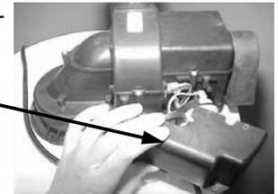
Step 3. Locate blower temperature switch.
