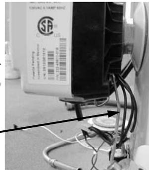
Step 7. Pivot the tool towards the water heater, as far as possible. Lift straight up on the gas control. The gas control should move about  $1/8$ ". Hold the gas control in position and remove the tool. Lift straight up on the gas control to remove it completely from the thermal well.
