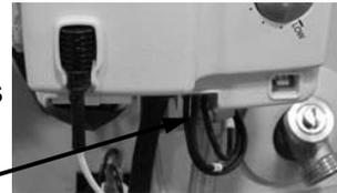
Step 2. With a multi-meter set to the ohms setting, measure the resistance between the middle and right side wires.
