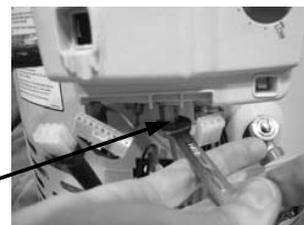
Step 8. Disconnect the spark igniter/flame sensor wire from gas control.
