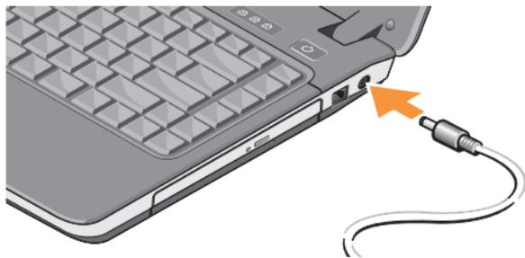
**CAUTION:** The AC adapter works with electrical outlets worldwide. However, power connectors and power strips vary among countries. Using an incompatible cable or improperly connecting the cable to a power strip or electrical outlet may cause fire or equipment damage.
