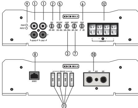
4 gauge power and ground wiring is recommended for all D3 amplifiers
