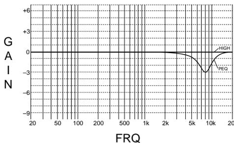
If you want to change the characteristics, follow the procedure below to adjust the frequency and gain for the high-shelving equalizer (HIGH) and parametric equalizer (PEQ). For the more detailed characteristics in different settings, see “CINEMA-EQ Frequency Characteristics” on page 82.
