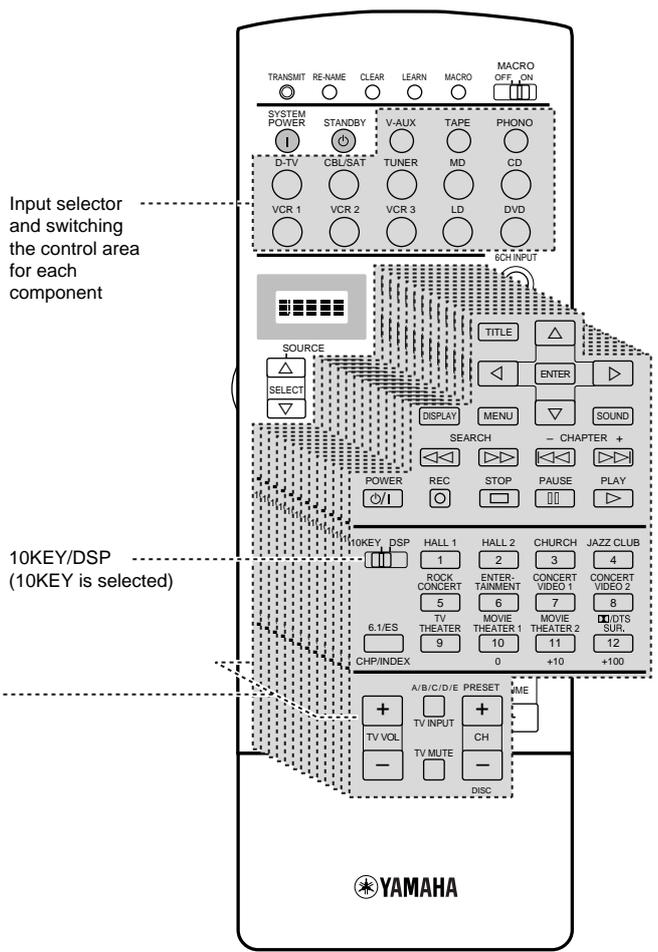
There are 14 component control areas. You can setup the manufacturer code and program other remote control functions in each area (Cannot setup the manufacturer code in the OPTN area). See pages 57 and 58.
