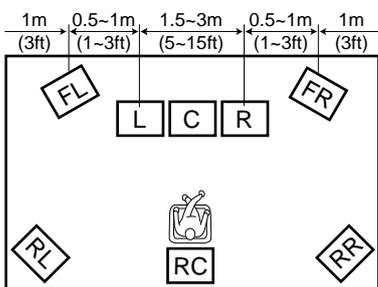
These speakers should be placed about 0.5~1m (1~3 feet) outside the Main speakers and in the front of the room. They should be turned toward the main listening position. Place the Rear speakers in the back of the room so they face the main listening position. The Rear speakers can be placed farther apart than the Front Effect speakers. The Front Effect and Rear speakers should be placed about 1.8m (6 feet) above the floor.
