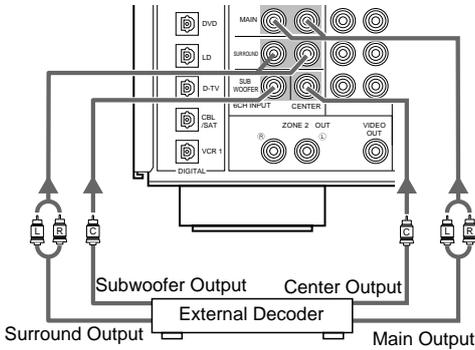
Connect the output jacks on your external decoder to the **6CH INPUT** jacks.
