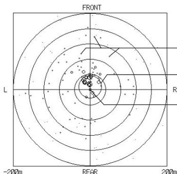
The center of these circles represent the virtual sound source. The size of the circle indicates the strength of the virtual sound source.
