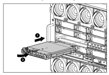
When installed in an operational enclosure, the switch automatically powers up and performs a series of Power On Self Tests.
