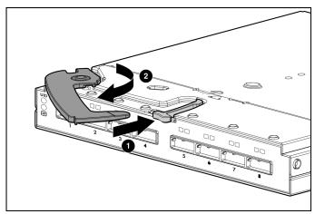
Install the switch in the open interconnect bay.
