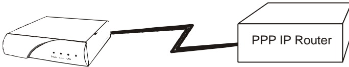
Figure 2 - 2 Basic PPP Leased Line Configuration
