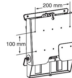
Fasteners for mounting unit to wall are customer supplied.
