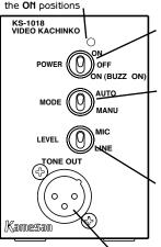
POWER switch: three settings: ON is on, with no buzzer, OFF turns the unit off, and ON (BUZZ ON) uses the built-in buzzer
