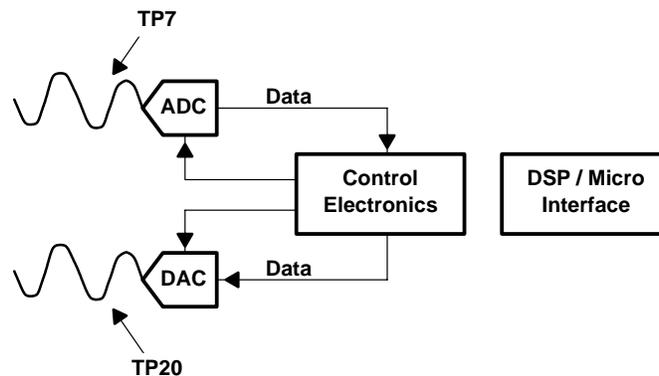
The user may probe the data and control signals to observe the signals that allow stand-alone mode to function.
